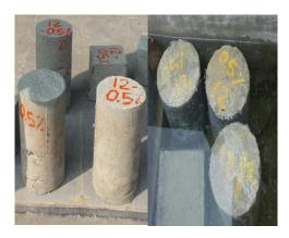
Cracks Developed On Cylinders After Load Applied
